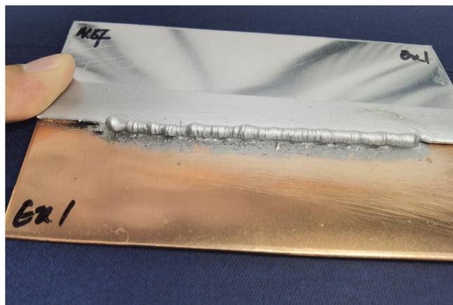
Figure.3 Best condition of TIG-MIG hybrid joining.
